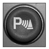
URPA can be turned off by pressing the rear park aid disable switch located near the climate control system and radio. You will not see any lights on the rear display if URPA is turned off.
